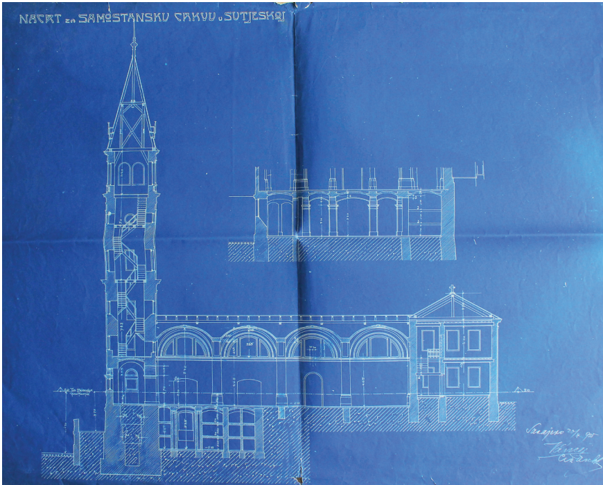
Figure 10. The Parish Church of Saint John the Baptist, Kraljeva Sutjeska: longitudinal section view through the eastern bell tower and the side aisle; a segment of the second project done by Josip Vancaš, dated on 20 th April 1905 36
